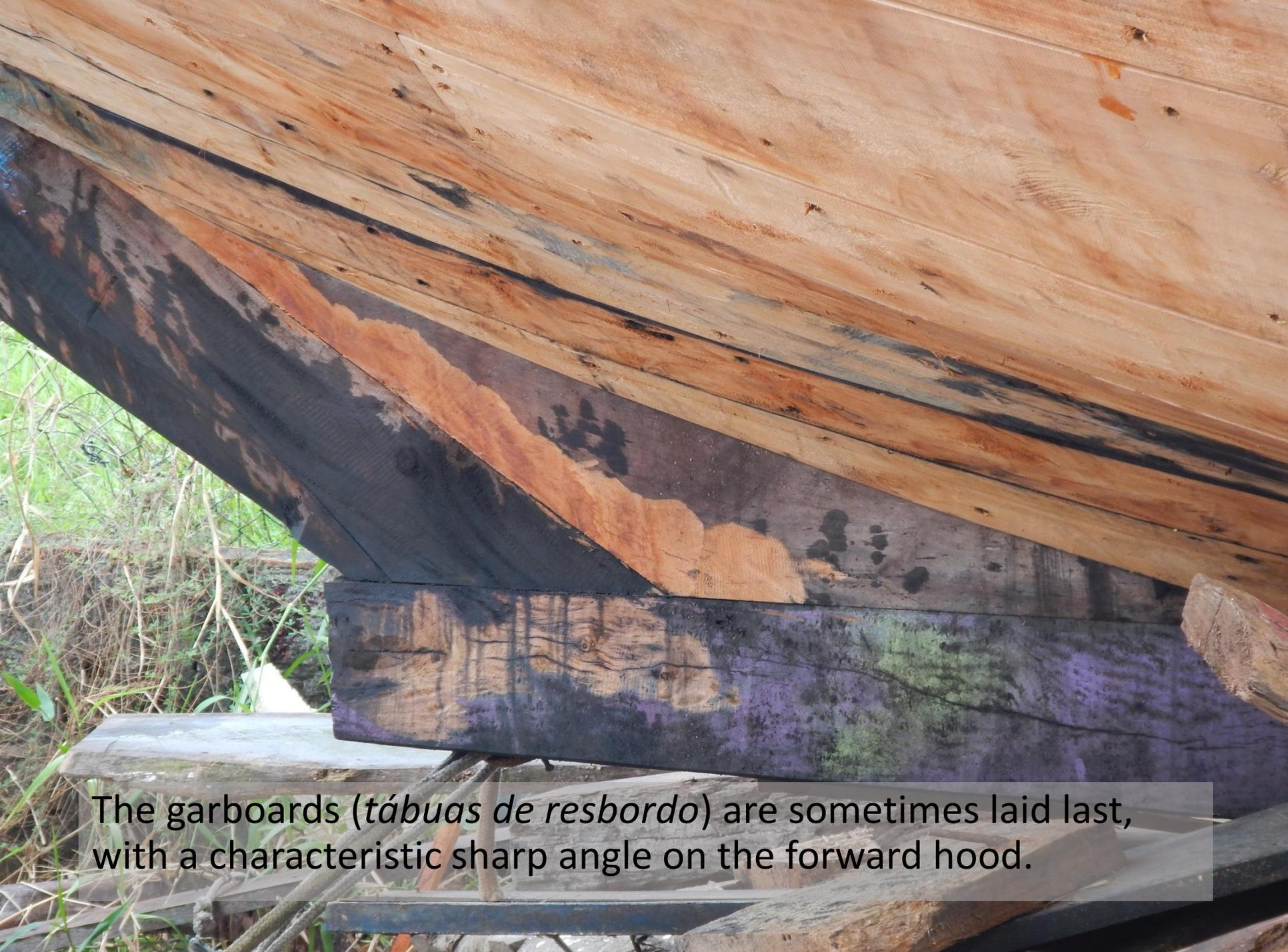
The garboards (*tábuas de resbordo*) are sometimes laid last, with a characteristic sharp angle on the forward hood.
