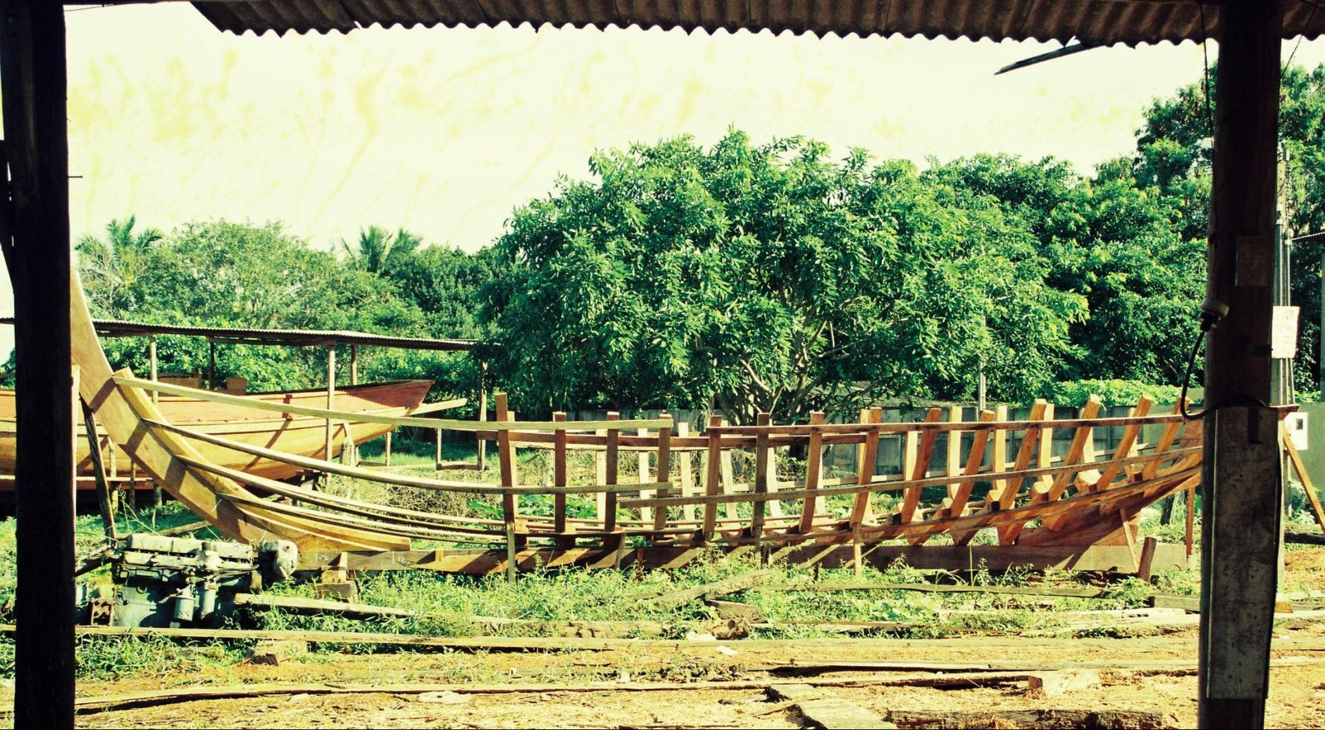
Building with master frames, gauges, and ribbands requires a certain period of apprenticeship to understand the use of geometric aids, which can be used without a full understanding of the geometric steps needed to design the molds, calculate the gauges, or determine the number of pre-designed frames.
