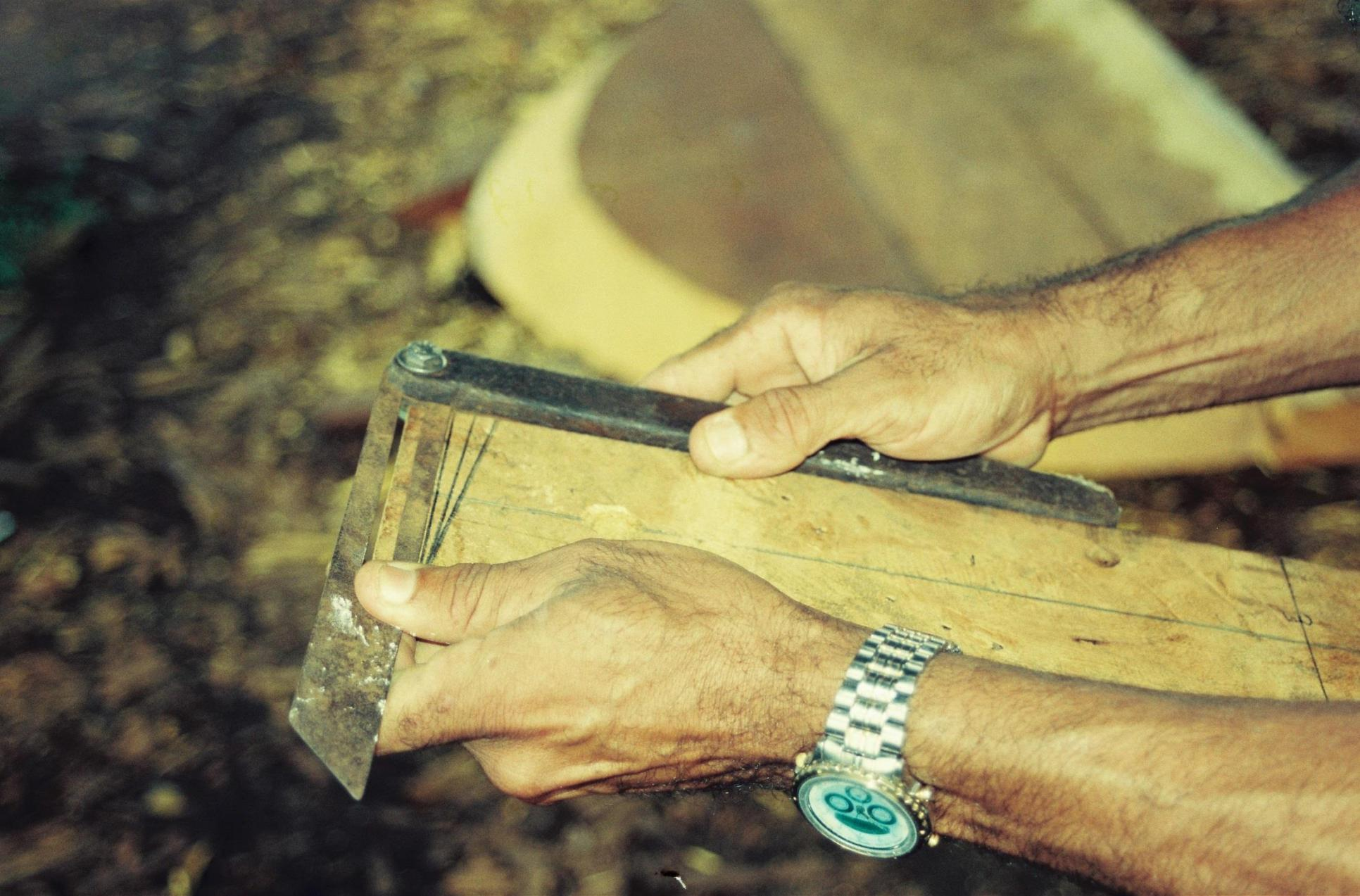
Bevels (*sotamentos*) are cut with the help of a scale marked in the *graminho*.
