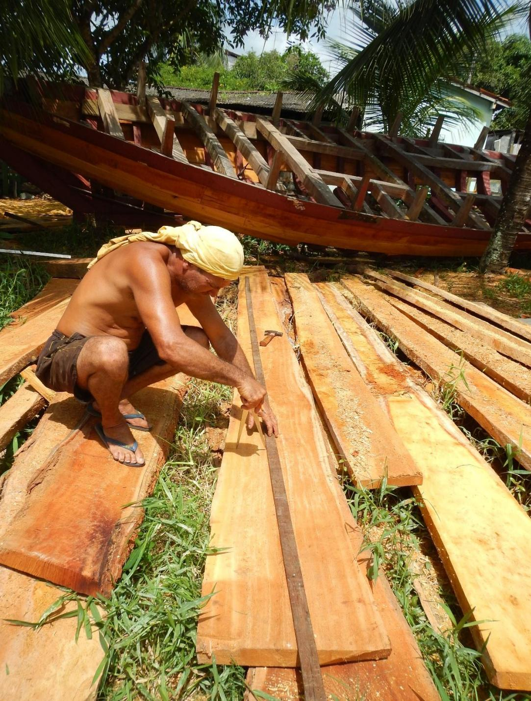
Spiling (*fasquilhar*) is done with a thin ribband (*fasquilha*), from which offsets are measured at each frame. The measurements are transferred to the inner face of the plank being shaped.
