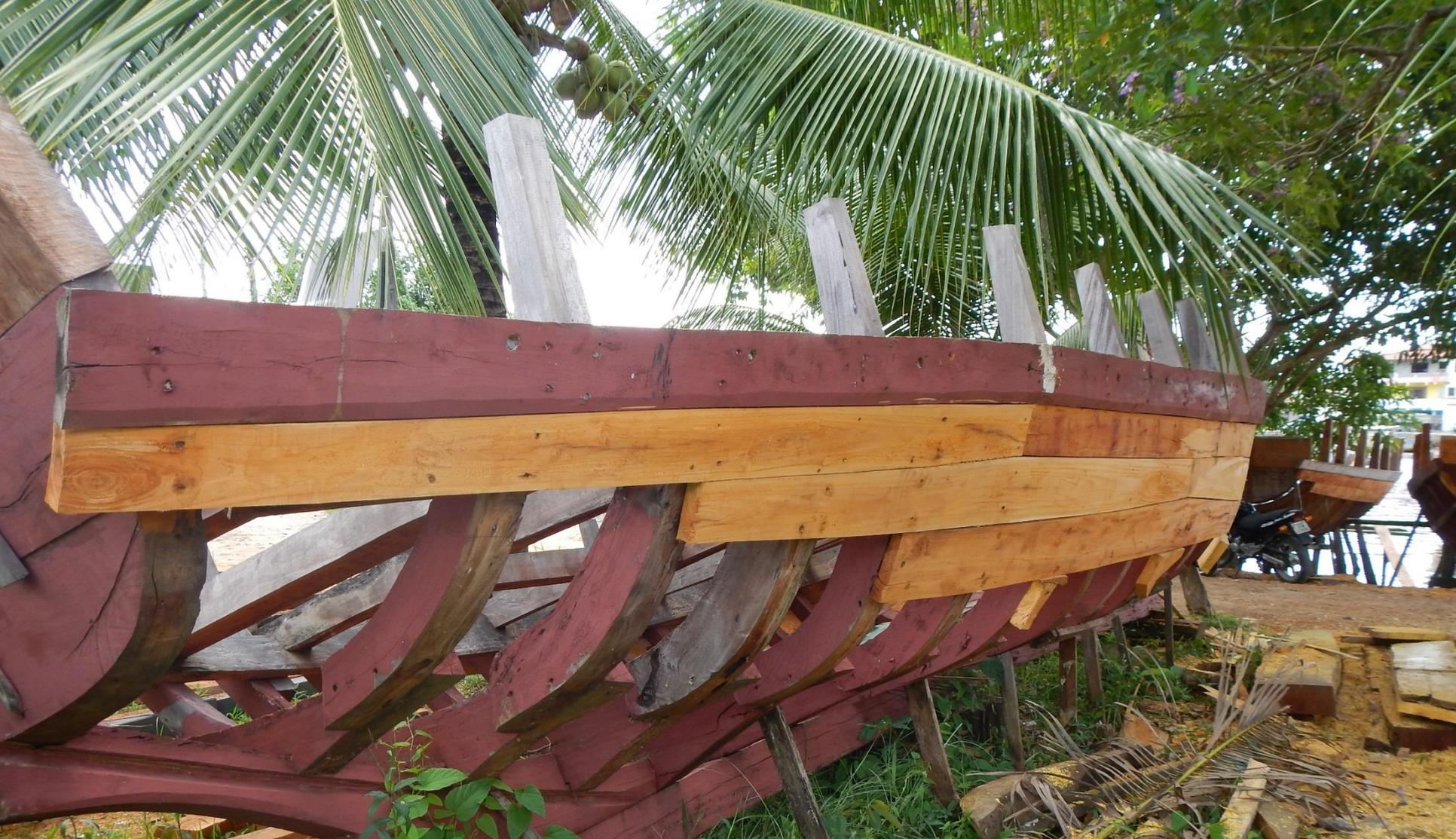
The main wale (*cinta*) is fastened to the complete framing, bent with the help of ropes and clamps, augured and fastened with screws – bolts in the past.
