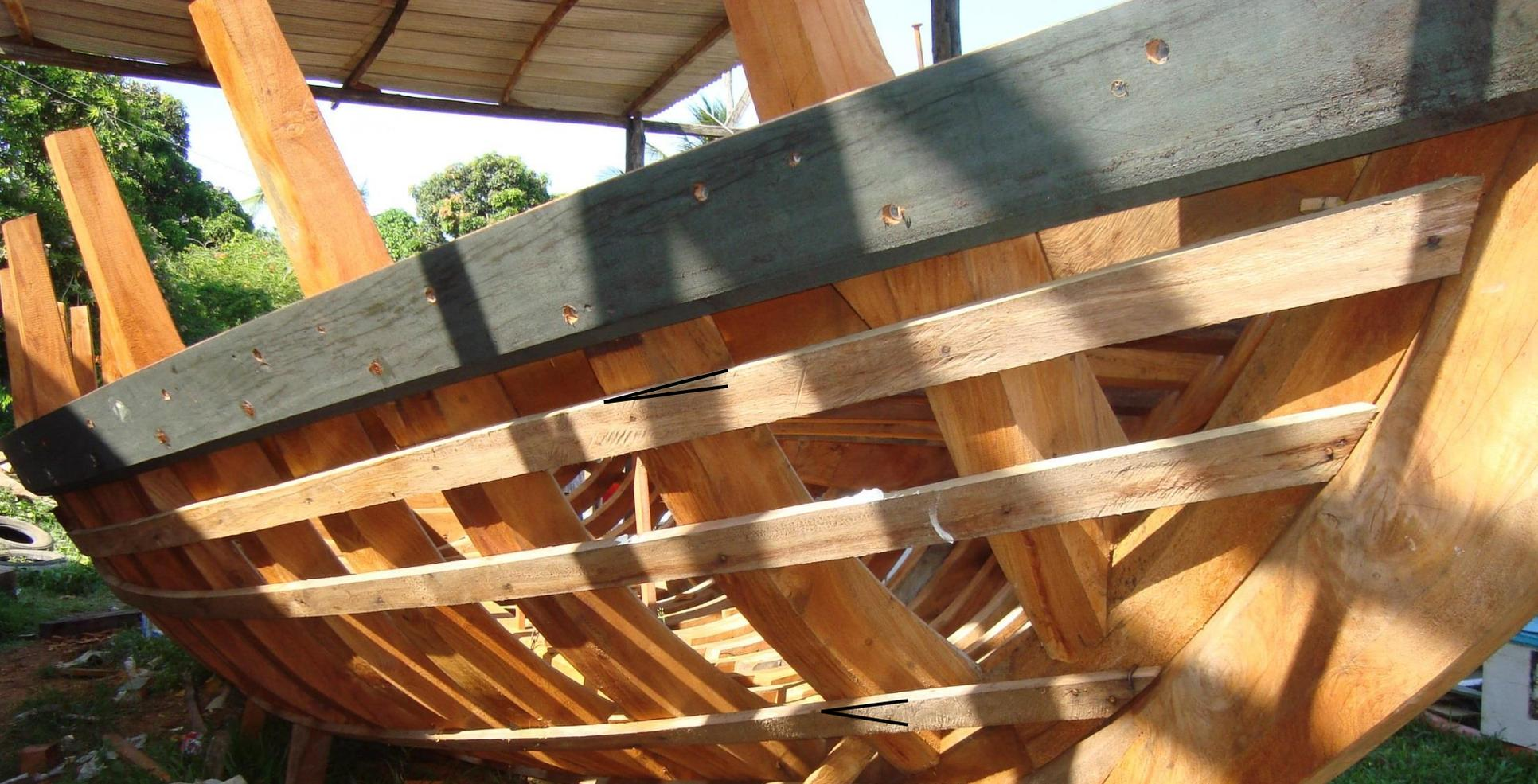
All bevels are marked with the help of a bevel gage (*suta*) at certain points along the length of the timbers and adzed out. The bevels seem to be measured directly from the *graminho* on the floor timber, but they are increased along the extension of the futtocks, being more pronounced on the top than the bottom sections.
