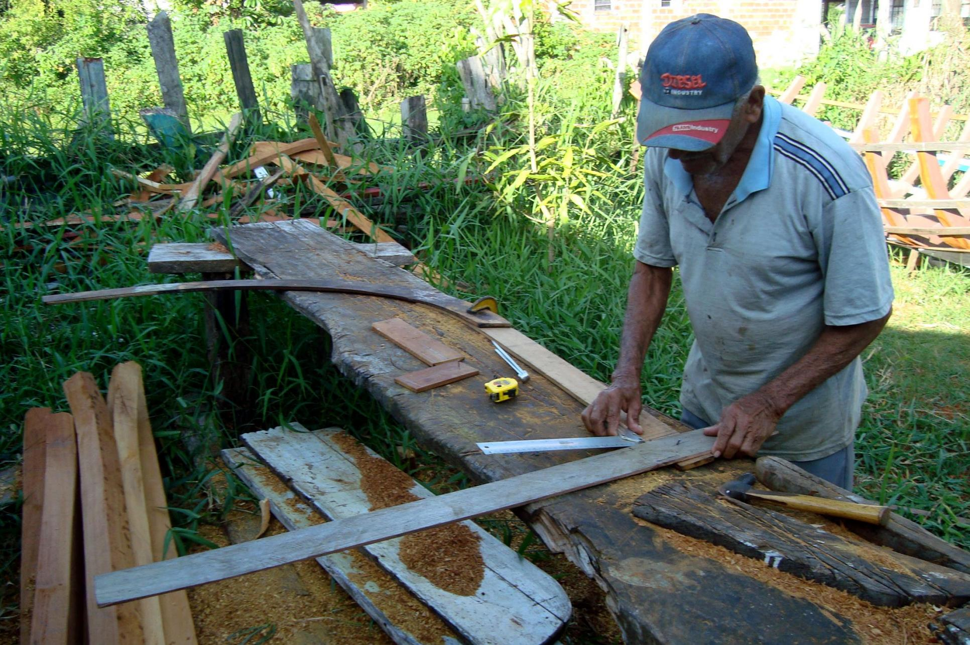
A small number of molds, gauges (*graminhos*), and ribbands are used to obtain – or repeat – a particular hull shape with reasonable accuracy.
