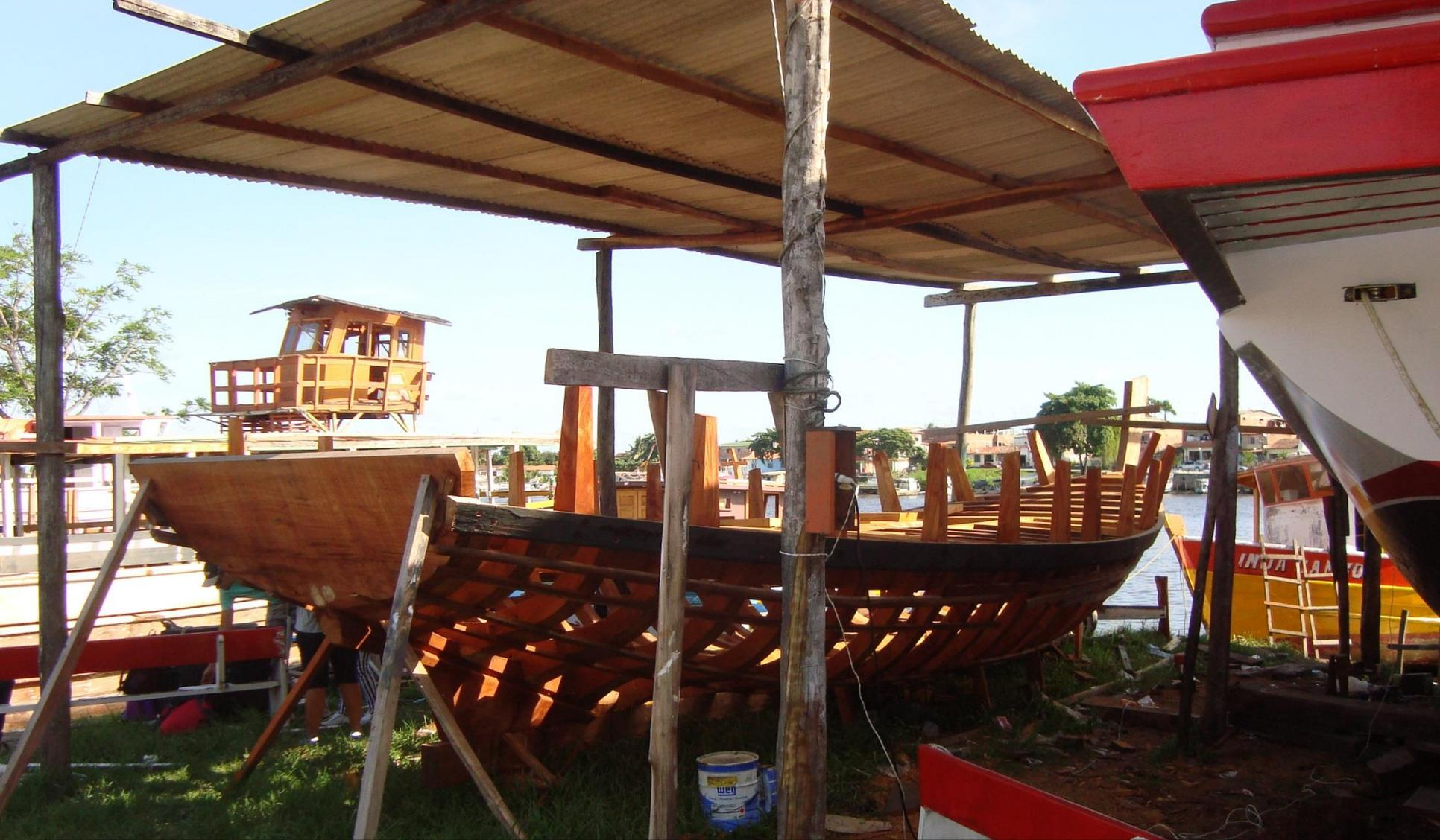
The stern panel, assembled with thick planks, is normally half as wide as the maximum beam and shaped with the futtock arcs inversed (with the turn of the bilge up).
