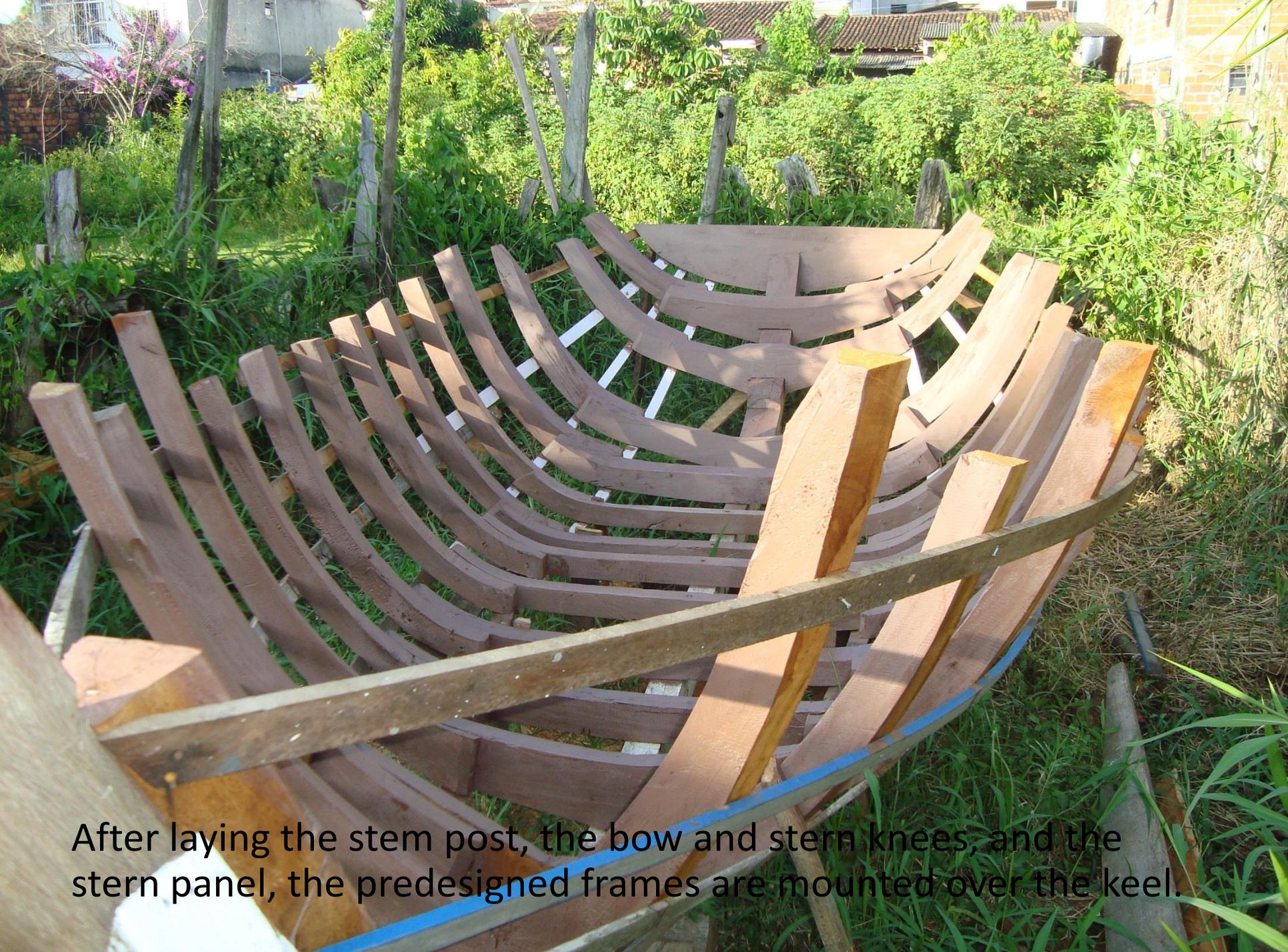
After laying the stem post, the bow and stern knees, and the stern panel, the pre-designed frames are mounted over the keel.
