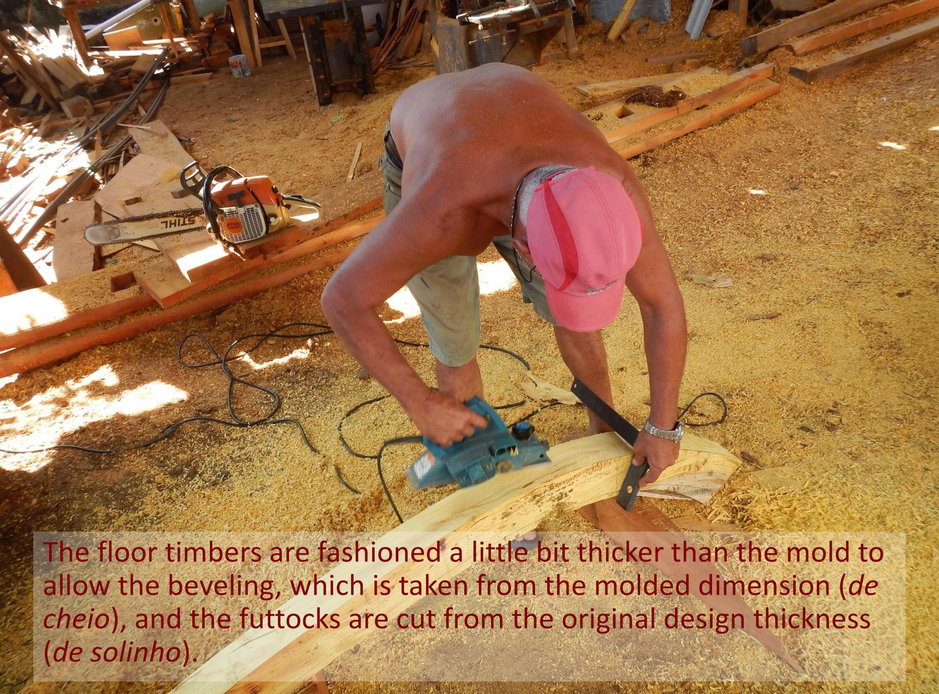
The floor timbers are fashioned a little bit thicker than the mold to allow the beveling, which is taken from the molded dimension (*de cheio*), and the futtocks are cut from the original design thickness (*de solinho*).
